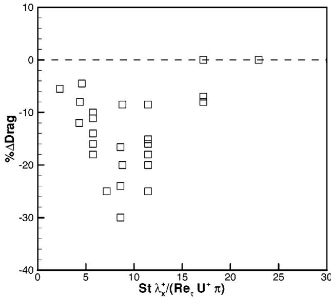
FIG. 22. Magnitude of Eq. (41),  $St \lambda_x^+ / (Re_\tau U^+ \pi)$ , compared to percent drag reduction for  $\Delta^+ = 10$ . It can be seen that a value of approximately 10 is most effective at reducing the drag.
