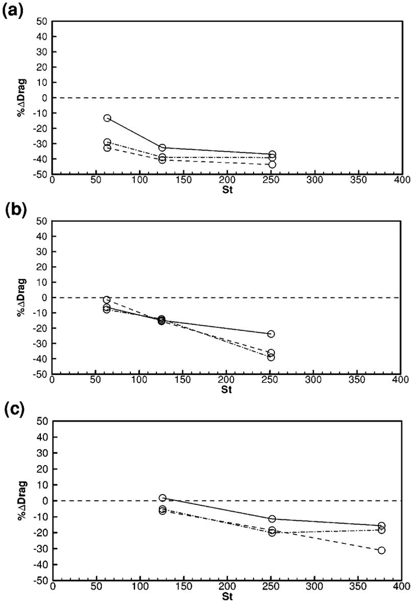
FIG. 10. Results of parametric study of drag reduction for oscillation frequency,  $T^+ = 50$ : (a)  $Re_\tau = 100$ ; (b)  $Re_\tau = 200$ ; (c)  $Re_\tau = 400$ . It can be seen that the  $St$  required to obtain the same amount of drag reduction increases with increasing  $Re_\tau$ , and that an optimal value of  $St$  exists for a given  $T^+$ :  $\Delta^+ = 5$ , —;  $\Delta^+ = 10$ , ---;  $\Delta^+ = 20$ , -.-.
