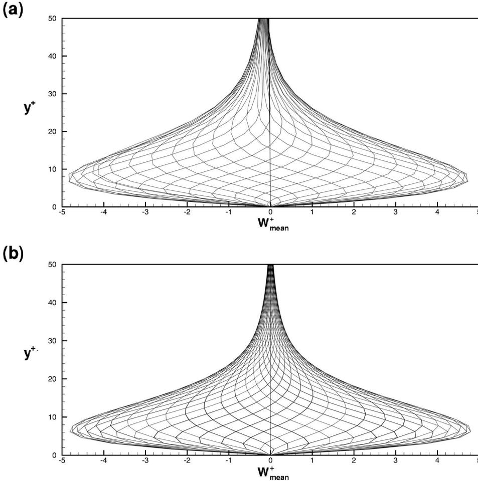
FIG. 9. Induced spanwise velocity profiles: (a) turbulent case; (b) analytical solution of Eq. (25). The different curves represent different instances in time during the forcing period.
