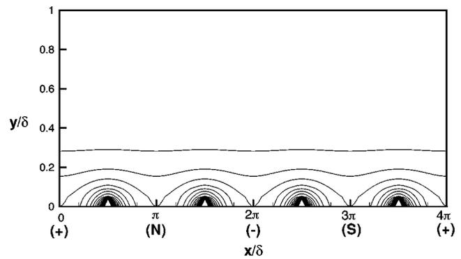
FIG. 14. Force distribution resulting from potential distribution representation in Fig. 13. Note that force is positive everywhere and contour values range from 2 to 40 [N] with 21 levels shown.
