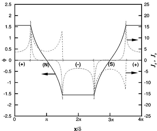
FIG. 13. Electric field potential  $\phi$  and current density  $\mathbf{J} = -\sigma \nabla \phi$  defined by step-function/tangent distribution. The variation of the magnetic field (not shown) is similar:  $\phi$ , —;  $J_x$ , ---;  $J_y$ , -.-.
