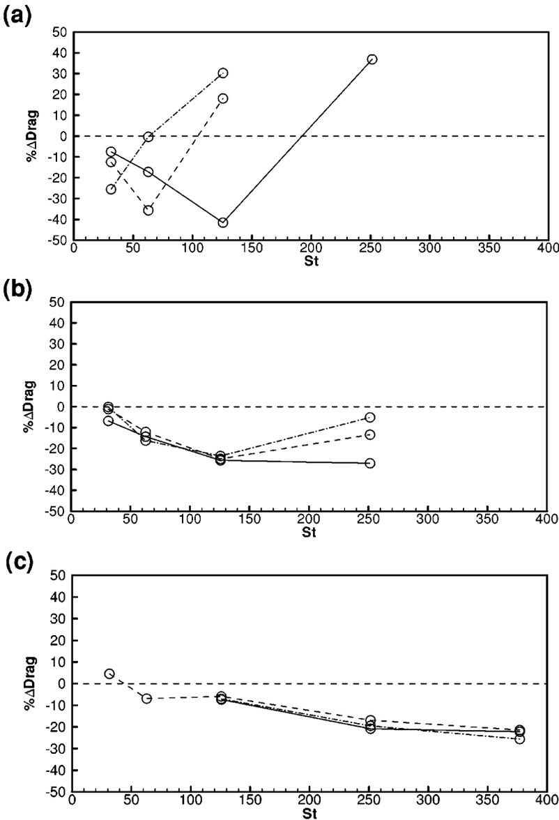
FIG. 11. Results of the parametric study of drag reduction for oscillation frequency,  $T^+ = 100$ : (a)  $Re_\tau = 100$ ; (b)  $Re_\tau = 200$ ; (c)  $Re_\tau = 400$ . It can be seen that the  $St$  required to obtain the same amount of drag reduction increases for increasing  $Re_\tau$  and that an optimal value of  $St$  exists for a given  $T^+$ :  $\Delta^+ = 5$ , —;  $\Delta^+ = 10$ , ---;  $\Delta^+ = 20$ , -.-.
