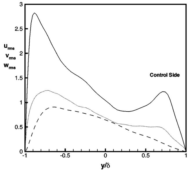
FIG. 7. Root-mean-square velocity fluctuations for a spanwise oscillating Lorentz force for  $Re_\tau=100$ ,  $St=20\pi$ ,  $\Delta^+=10$ , and  $T^+=100$ :  $u_{\text{rms}}/u_\tau$ , —;  $v_{\text{rms}}/u_\tau$ , ---;  $w_{\text{rms}}/u_\tau$ , ...-. The rms values are normalized by  $u_\tau$  of the uncontrolled channel.
