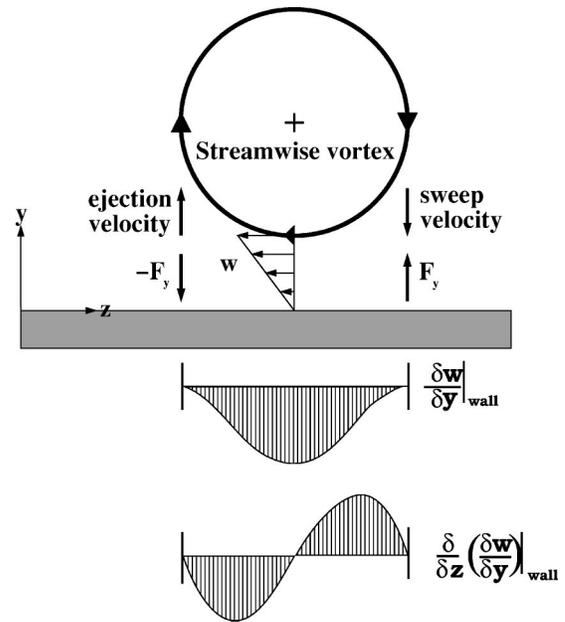
FIG. 24. Control scheme to detect and suppress near-wall streamwise vortices (Choi *et al.*<sup>17</sup>). Both the spanwise shear stress profile and corresponding spanwise shear stress gradient at the wall are shown.
