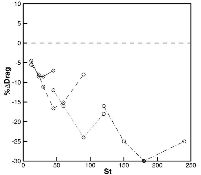
FIG. 17. Drag comparison for a spatially varying spanwise Lorentz force for  $\lambda_x^+ = 300, 600, 1200, 2400, \Delta^+ = 10$  and  $Re_\tau = 200$ , again revealing that there is an optimal  $St$  for each streamwise wavelength. In addition, there appears to be an optimal wavelength for producing maximum drag reduction:  $\lambda_x^+ = 2400$ , —;  $\lambda_x^+ = 1200$ , ---;  $\lambda_x^+ = 600$ , -.-.;  $\lambda_x^+ = 300$ , ....
