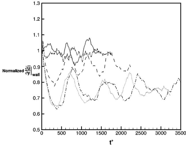
FIG. 19. Drag history for  $\lambda_x^+ = 300$  and  $\text{Re}_\tau = 100$  illustrating the existence of an optimal  $\text{St}$ : no control, —;  $\text{St} = 60$ , ---;  $\text{St} = 90$ , - · -;  $\text{St} = 120$ , ···;  $\text{St} = 180$ , - · - · -.
