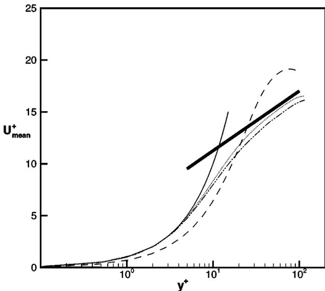
FIG. 6. Mean velocity profile on the control side of the channel in terms of wall units for a spanwise oscillating Lorentz force for  $Re_\tau=100$ ,  $\Delta^+=10$ : no control, ...;  $u^+=y^+$ , —;  $u^+=2.5 \ln(y^+)+5.5$ , —;  $St=20\pi$  and  $T^+=100$ , ---;  $St=4\pi$  and  $T^+=500$ , -.-.-.
