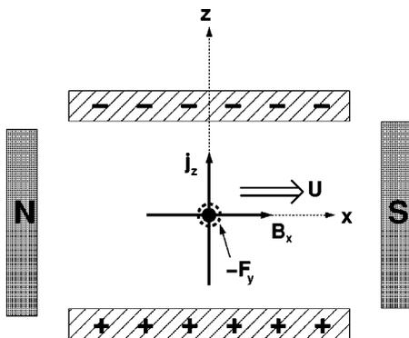
FIG. 23. Electrode and magnet configuration that produces a significant wall-normal force (Nosenchuck and Brown<sup>7</sup>).
