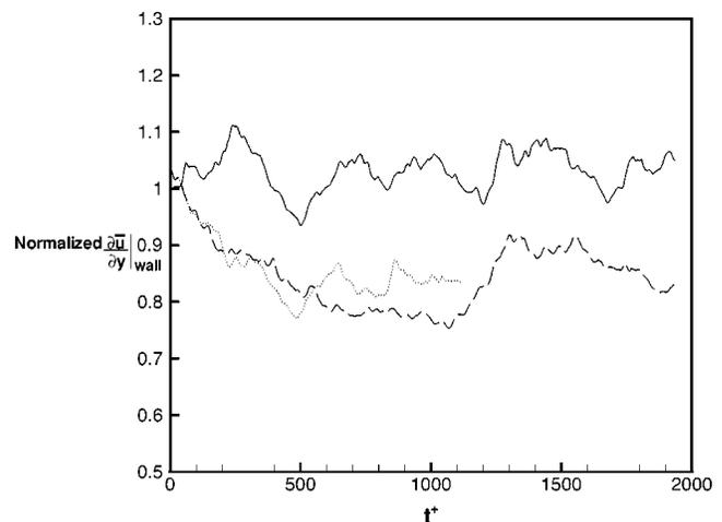
FIG. 15. The drag history comparison between realistic and ideal force distributions for  $Re_t = 100$ ,  $\Delta^+ = 10$ , and  $St = 10\pi$ . No statistically significant difference can be discerned between the two cases: no control, —; realistic case,  $\cdots$ ; ideal case, ---.
