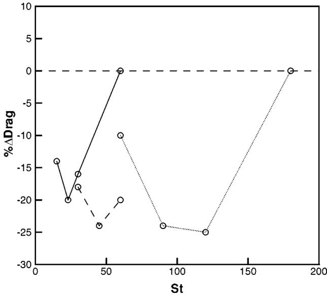
FIG. 16. Drag comparison for a spatially varying spanwise Lorentz force for  $\lambda_x^+ = 300, 600, 1200, \Delta^+ = 10$  and  $Re_\tau = 100$ , illustrating that there is an optimal  $St$  for each streamwise wavelength:  $\lambda_x^+ = 1200$ , —;  $\lambda_x^+ = 600$ , ---;  $\lambda_x^+ = 300$ , ....
