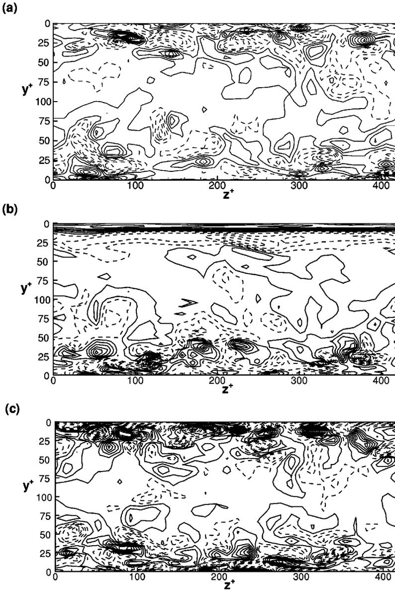
FIG. 4. Contours of streamwise vorticity,  $\omega_x$ , shown for  $Re_\tau=100$ : (a) no control; (b)  $T^+=100$ ,  $\Delta^+=10$ ,  $St=20\pi$ ; (c)  $T^+=500$ ,  $\Delta^+=10$ ,  $St=20\pi$ . Note that for  $T^+=100$  the streamwise vortices are nearly completely suppressed. Dashed lines indicate negative values. (Lorentz force applied at top wall only.)
