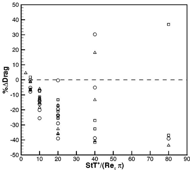
FIG. 12. Magnitude of Eq. (34),  $St T^+ / (Re_t \pi)$ , compared to the amount of percent drag reduction. For the cases considered, it can be seen that a value of 20 is most effective at reducing the drag:  $\square$ ,  $\Delta^+ = 5$ ;  $\triangle$ ,  $\Delta^+ = 10$ ;  $\circ$ ,  $\Delta^+ = 20$ .
