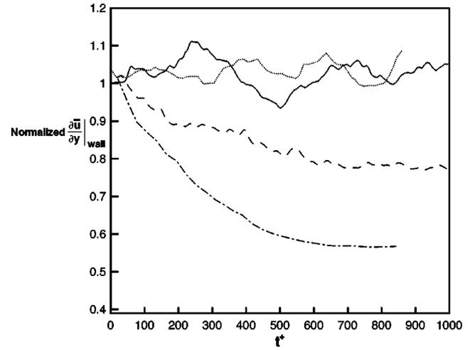
FIG. 3. Drag histories for  $\text{Re}_\tau = 100$  channel with  $\Delta^+ = 10$ : no control, —;  $T^+ = 100$  and  $\text{St} = 10\pi$ , ---;  $T^+ = 100$  and  $\text{St} = 20\pi$ , - · - ·;  $T^+ = 500$  and  $\text{St} = 20\pi$ , ···.
