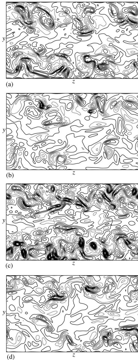
FIG. 4. Contours of streamwise vorticity in  $y$ - $z$  plane for  $L_s=0.02$ : (a) regular channel; (b) Case 1; (c) Case 2; (d) Case 3. Contour levels are from  $-100$  to  $100$  in increments of  $10$ .
