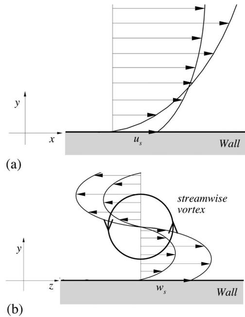
FIG. 5. A schematic representation of drag decrease and increase mechanism: (a) drag decreases with a streamwise slip velocity ( $x$ - $y$  plane); (b) drag increases with a spanwise slip velocity ( $y$ - $z$  plane).
