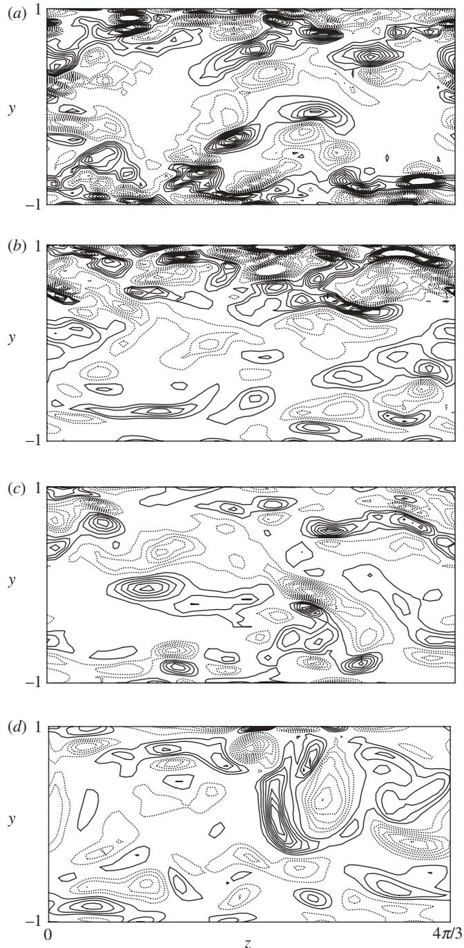
Figure 1. Contours of streamwise vorticity in the  $y$ - $z$  plane: (a) regular channel; (b) channel with an LQR controller on the bottom wall (T. Min 2005, unpublished data); (c) channel with a hydrophobic surface on both walls [8]; and (d) channel with a polymer [6]. Contour levels are from  $-1$  to  $1$  in increments of  $0.1$ .
