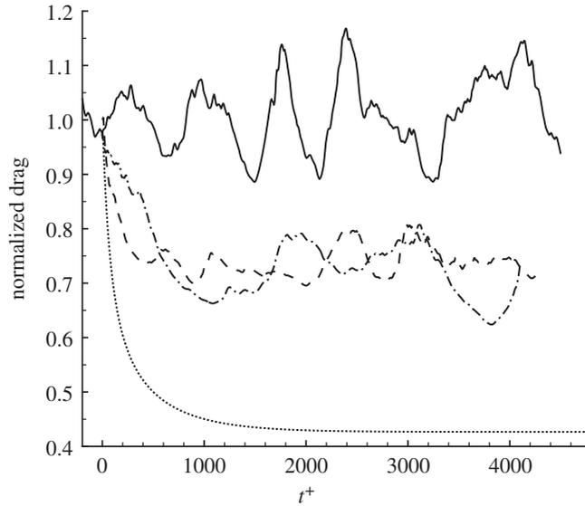
Figure 4. Mean skin-friction drag history with various control methods: solid line, no control; dashed line, opposition control ( $y_d^+ \approx 15$ ); dashed-dotted line, LQR control; dotted line, virtual flow.
